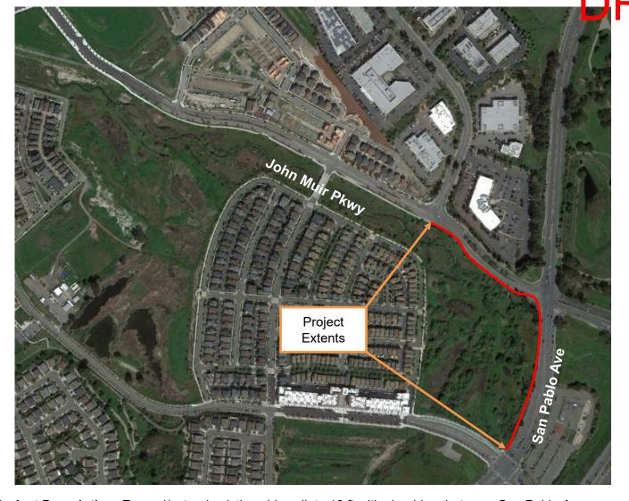
**Project Description:** Expand/extend existing sidewalk to 10 ft with shoulders between San Pablo Avenue and ITC. Install 10 ft sidewalk with metal railing and retaining wall along San Pablo Ave between Sycamore Avenue and John Muir Parkway.
