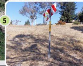
Underground Utilities 24" PG&E natural gas and 36" EBMUD water line located within City of Hercules parcel. New bridge and approach roadway should avoid these major utilities.
