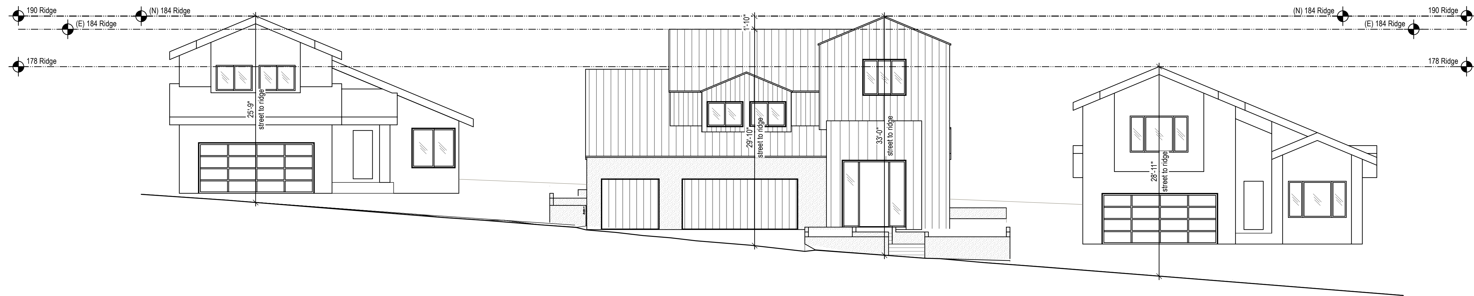
3 Proposed North Site Elevation scale: 1/8"=1'-0"
